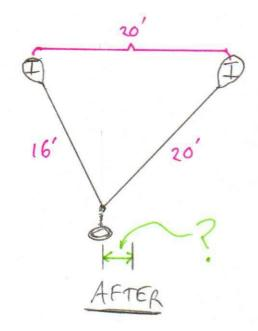
PROBLEM: A Rigger is told to change an even bridle by removing 4' of material out of the leg on the left side.
